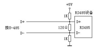
The 120  $\Omega$  resistances in the picture is terminal resistance. They are to prevent the signal reflection in the line. 1 K resistances are the level-pull-up resistor and level-pull-down resistor respectively. Its role is to ensure the line is logic "1" when the line is in leisure so that the data bits in cease - to prevent the reception error.
