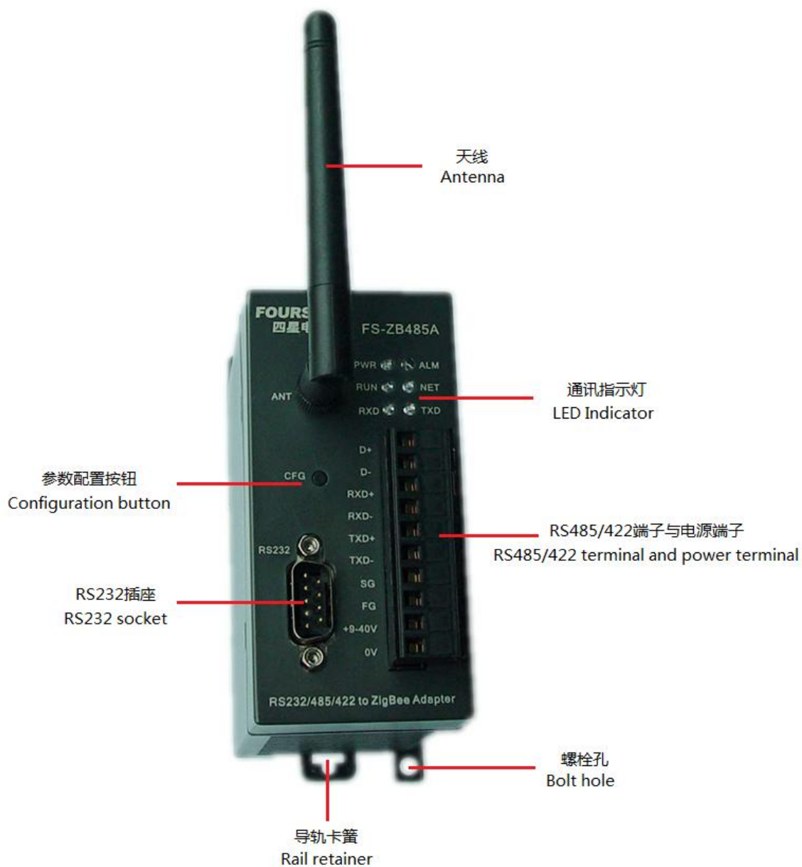
Figure 3-1 External structure and description of parts for FS-ZB485A
