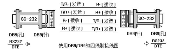
Notated, RXD, GND, COM as the basic four-signal system is have to be received in the figure above, and other signals in accordance with your product model.
