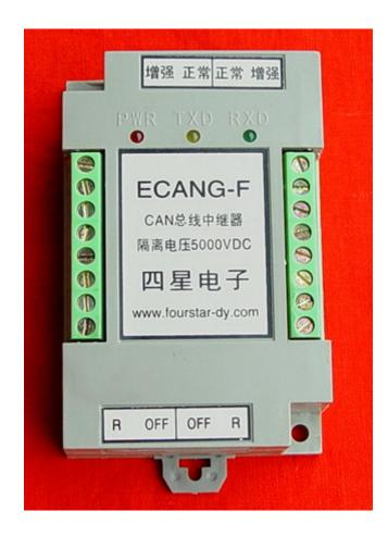
CAN optical isolated repeaters suit for explosion-proof area such as coral mine with high isolated voltage, which is 5000VDC or 3500VAC, can be used as intrinsically safe CAN repeaters when connected with intrinsically safe power supply externally and used in the intrinsically safe system in coral mine. Other functions are same as ECANG.
