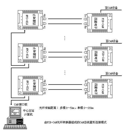
Fiber repeaters and fiber mode converters composed by FIB-CAN
