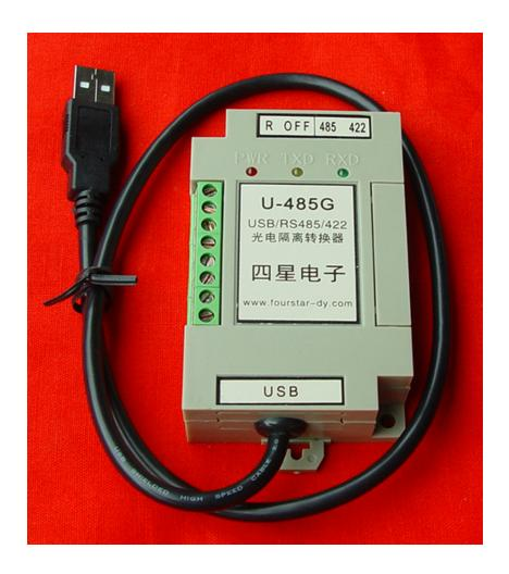
User's Guide for U-485G USB-RS485/422 high-speed light-isolated converters
