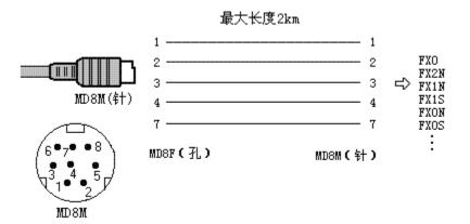
Due to internal resistance have been installed in USB-SC09-FX and the PLC, no external terminal resistance is needed.
