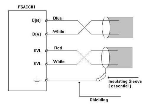
FSACC01 can make 64 PLC nodes form isolated RS485 communication network, the largest communication range is up to 2km (9600 bps), 3km(4800 bps), and without changing the existing communication software, as shown below. Turn the terminal resistance setting switch S2 on the FSACC01 of network's two ends to "R" (connect terminal resistance), the terminal resistance setting switch S2 of other nodes to "OFF" (don't connect terminal resistance).
